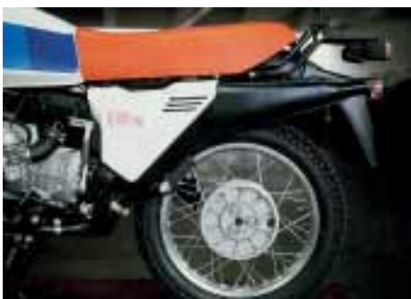
The revolutionary single swinging arm of the BMW R 80 G/S: wheel changing made simple.
