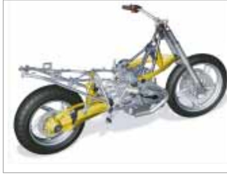
Far left: Drawing of the frame of the BMW R 1150 GS and, next to it, the BMW R 1200 GS with its Paralever placed overhead.
