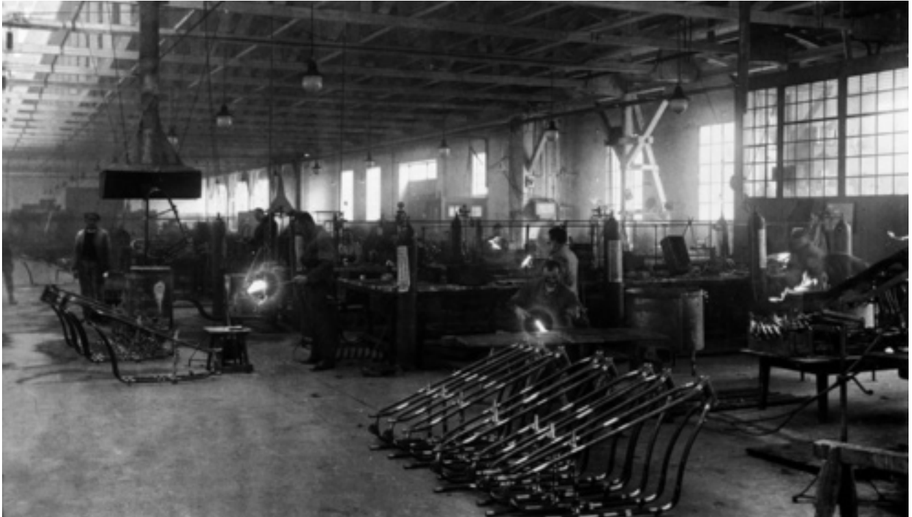
Above | Frames for the R 32, BMW's first motorcycle, being manufactured at the Munich factory in 1923.
