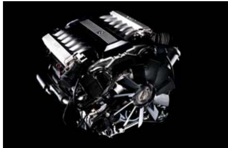
Above | The engine in the BMW 750i of 1987 was the first German-built 12-cylinder unit since the 1930s.
