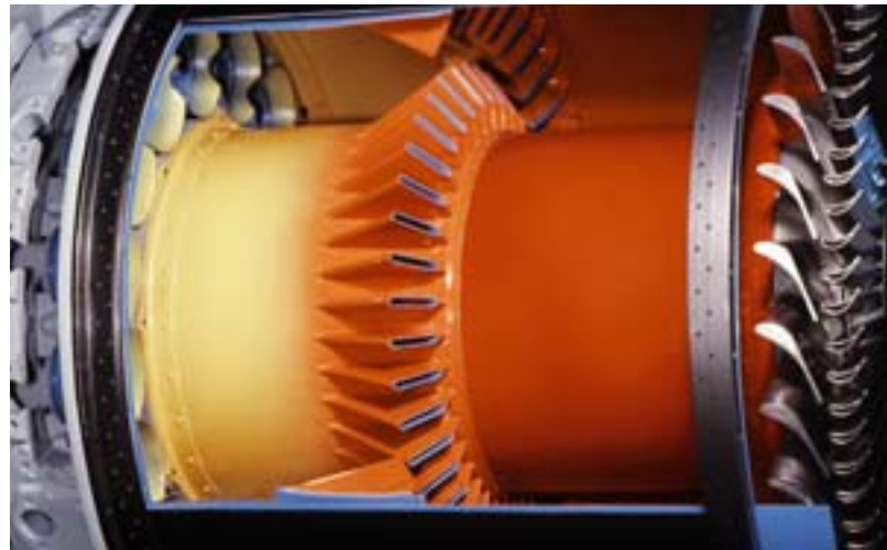
Above | View inside a BMW 003 unit. Visible from left to right: combustion chamber with air blending fins, cooling stators and turbine, 1978.
